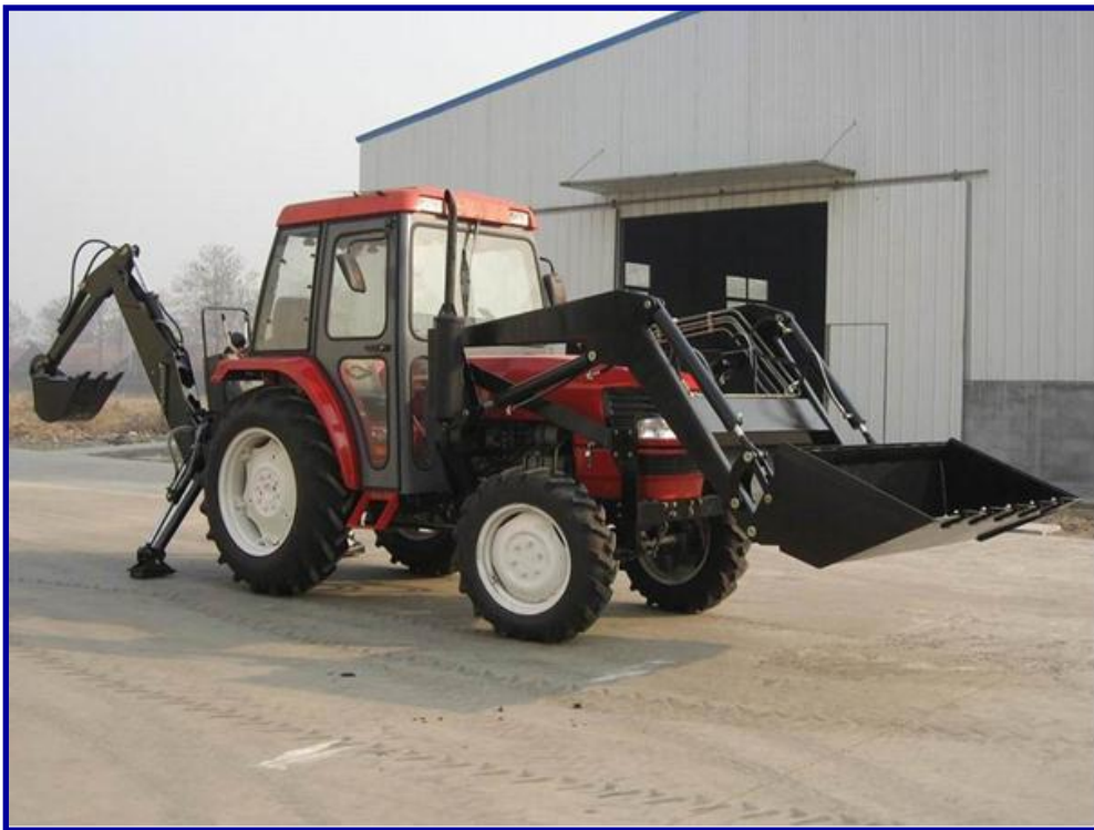
Figure 6 – Front end loader and backhoe attachments
