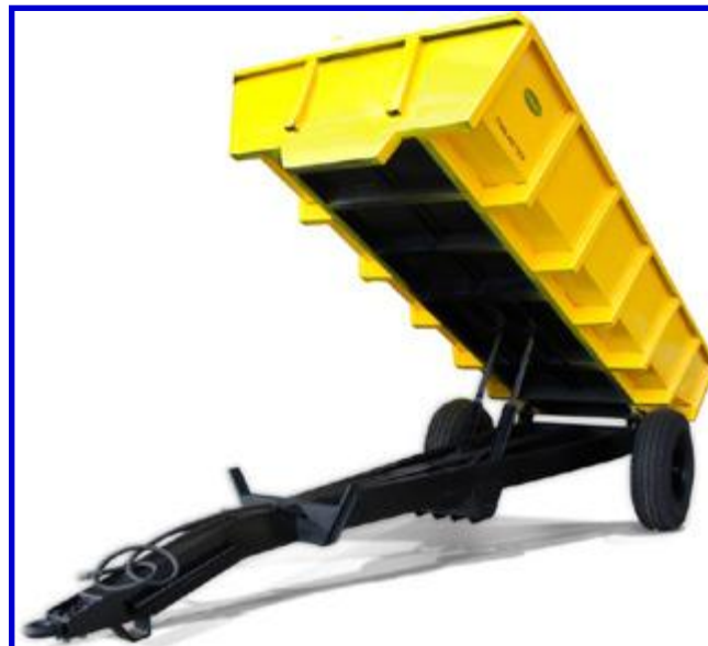
Figure 9 – 8 tonne Tipping Trailer (Landmech), South Africa
