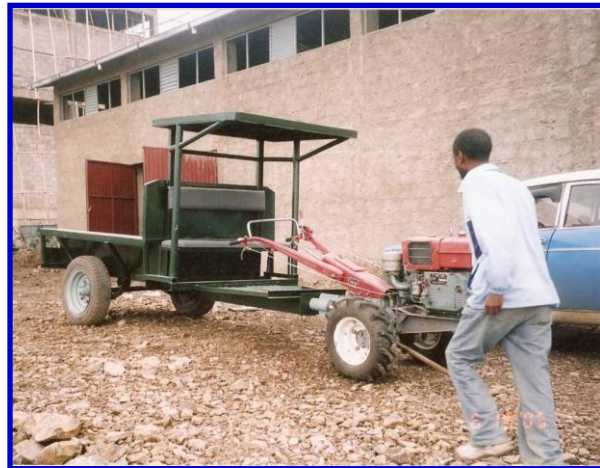
Figure 10 – General purpose trailer for Single Axle Tractor (Hebziba), Ethiopia
