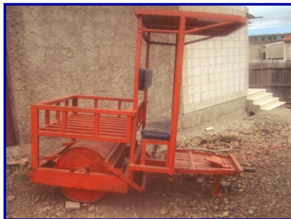
Figure 11 – Towed roller for Single Axle Tractor (Hebziba), Ethiopia
