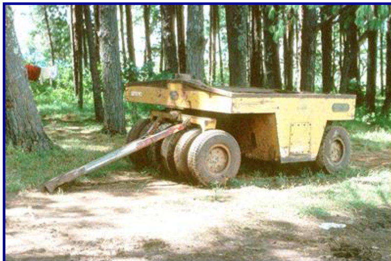
Figure 14 – Towed Pneumatic Tyred Roller (PTR)
