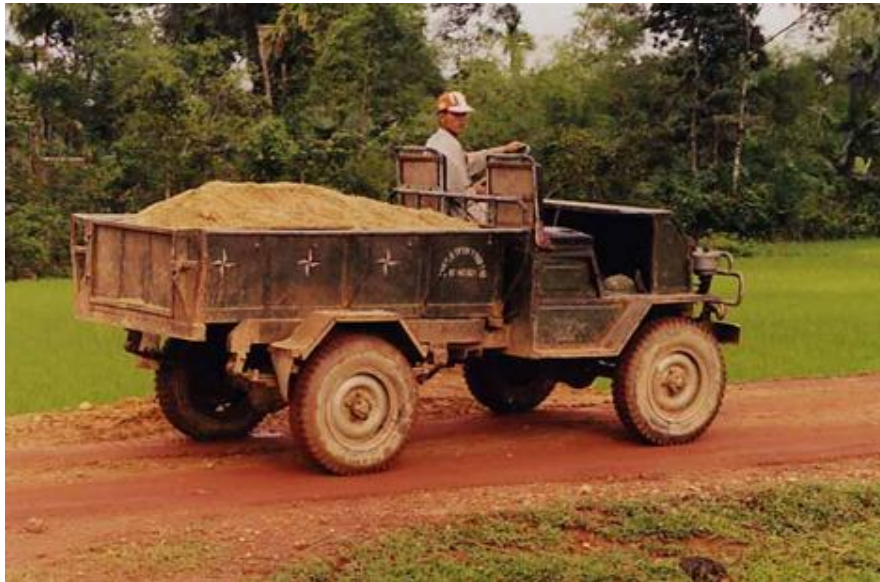
Figure 18 – Locally made 4WD Small Rural Vehicle (SRV) (Vietnam)
