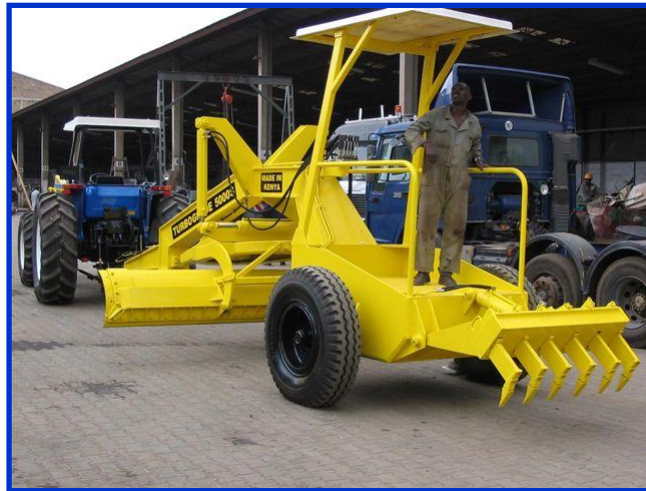
Figure 3 – Tractor and 5 tonne heavy towed grader (CMC), Kenya
