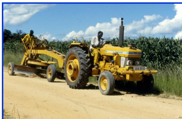
Figure 5 – Tractor and 2 tonne towed grader (Arthur Garden), Zimbabwe
